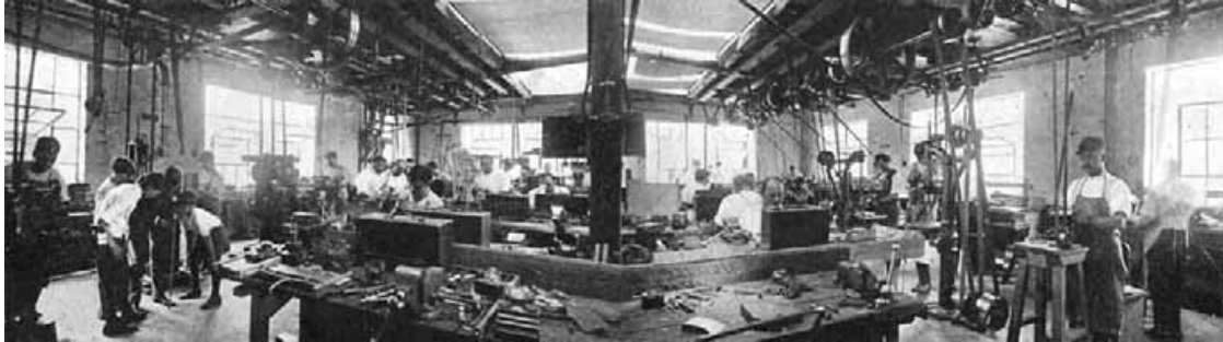
The tool-making room on the second floor of the first phase of the Irvington factory in 1917, notable for its overhead drive shaft and pulleys. This view looks directly through the center windows to South 21 st Street. Tool making was a critical first step in fabricating tools and dies needed to manufacture components for Lionel. The size of this operation relative to the overall factory attested to the priority the company gave to precision tooling.
